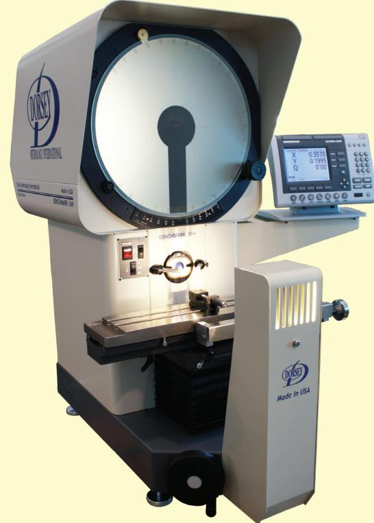
*This ultra precision system utilizes an integrated zero backlash, high resolution scale, in a free state, normalized zero stress stage. These features combine to attain inherent accuracy and repeatability values as high as +/- .000025" without electronic compensation.*
